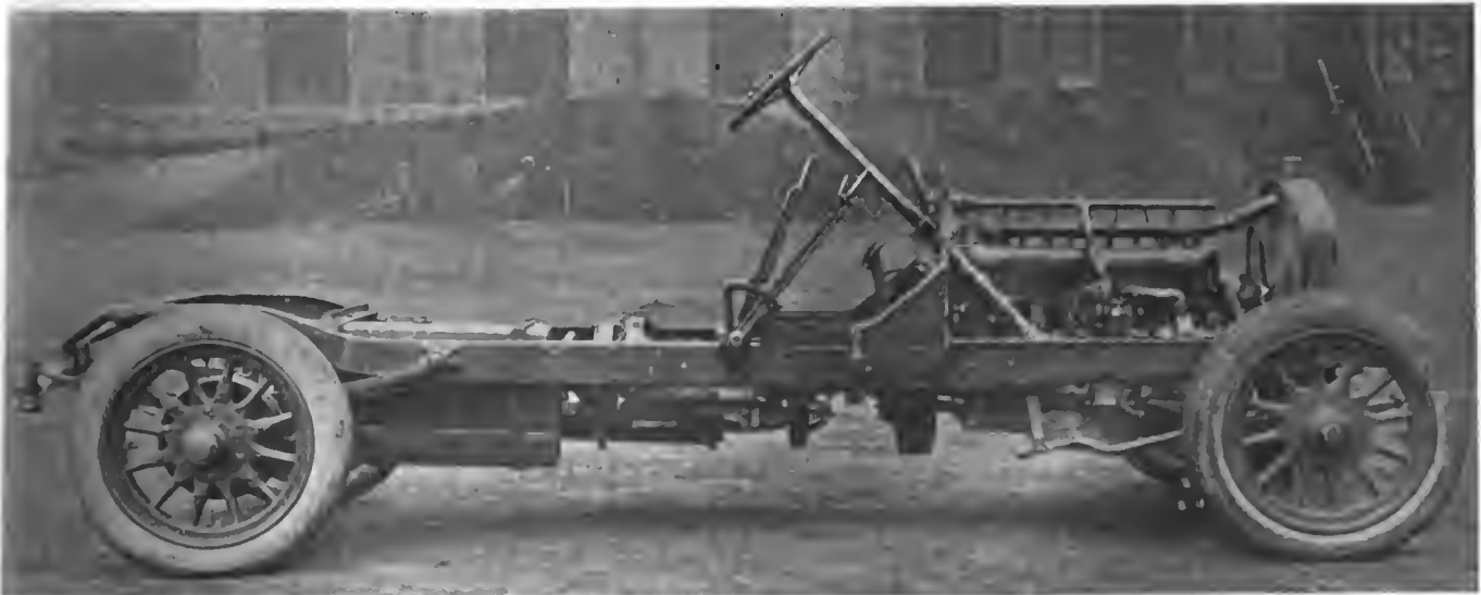
40-50-Horsepower Wolaeley with 6 Cylinders Cast in a Block and Applied Sheet Metal Jackets
